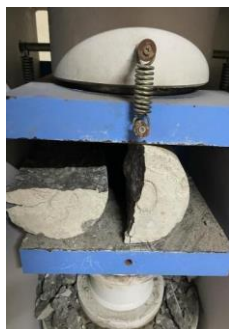
Fig. 5. SPLIT TENSILE TESTING
